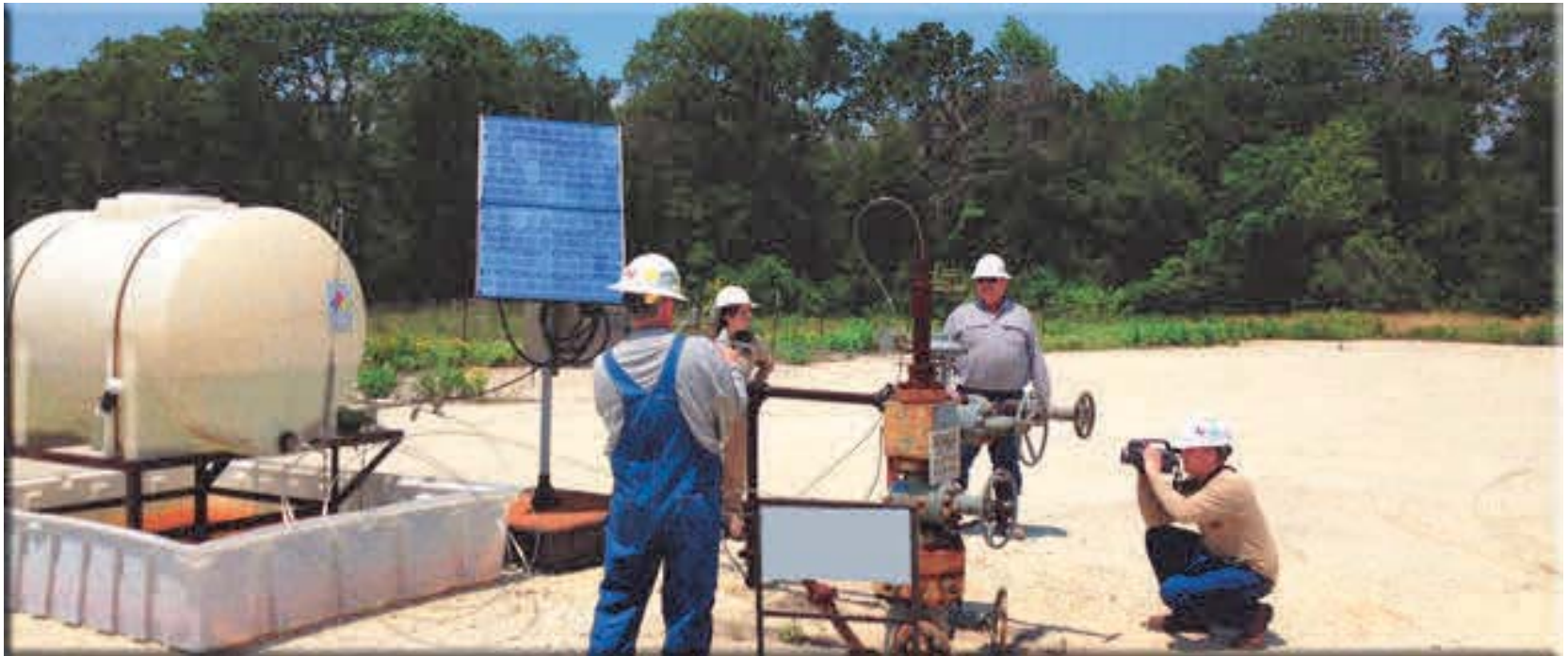
Optical Gas Imaging Camera being used to scan a wellhead for leaks (Source: University of Texas)
